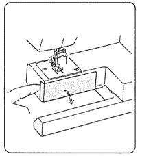
Remove the extension table from the machine by pulling it to the left. Open the shuttle cover by pulling down the embossed part on the left side of the cover.
